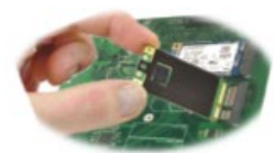
miniPCIE Expansion Slot
